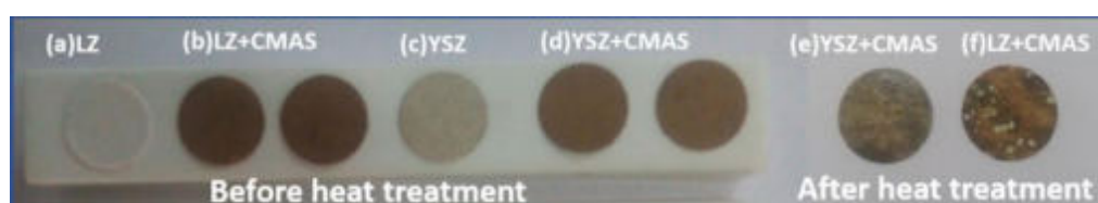
Fig. 1 (a) Free standing coating of LZ (b&c) LZ coating loaded with CMAS (c) free standing YZ coating (d) YZ coating loaded with CMAS (e) YSZ coating after reacting with CMAS (f) LZ coating after reacting with CMAS
